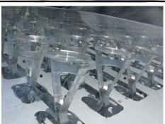
Left: Close up of Parans sun tracking lenses. The lower focusing element glows as the upper Fresnel lens directs the sun light to it
